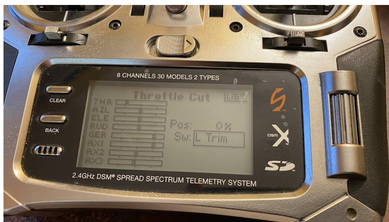
Spektrum DX8 Throttle Cut setup menu
