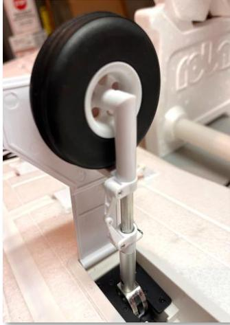
*Simulated OLEO suspension is just one of the many scale features on the T-28*
