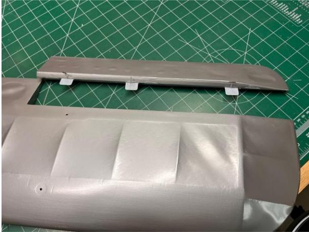
The left lower aileron was misaligned with glued at the factory. The original hinges had to be cut and new hinges installed so the aileron would have full deflection.
