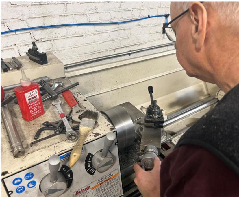
*Machining the exhaust valve using the lathe*
