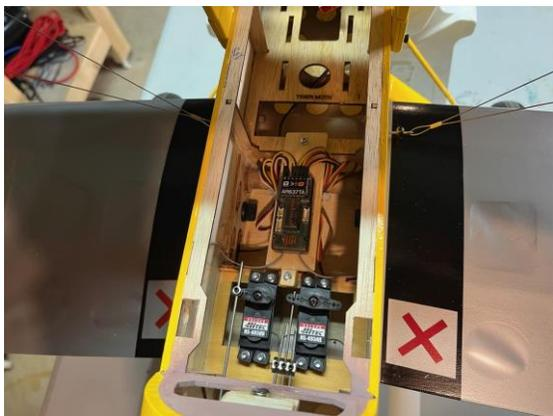
A mounting plate was made to make it easier to install the receiver and tidy up the wires. Two Hitec standard servos were used for the elevator and rudder.
