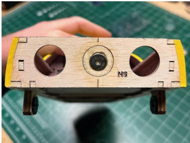
One of the holes in the hatch was filled in with a magnet mount.
