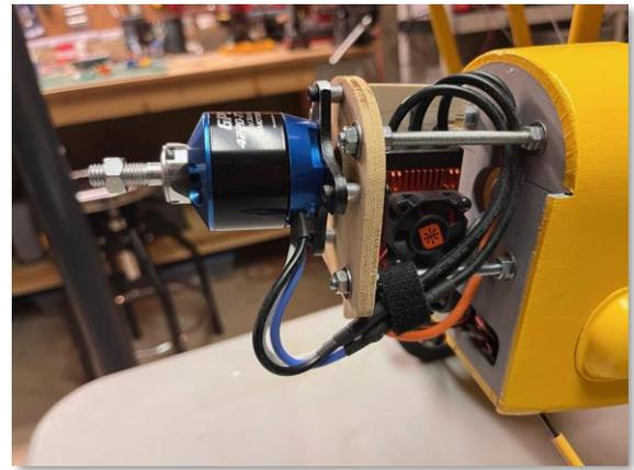
The ESC is tucked in front of the firewall and should add some needed weight to balance the center of gravity.
