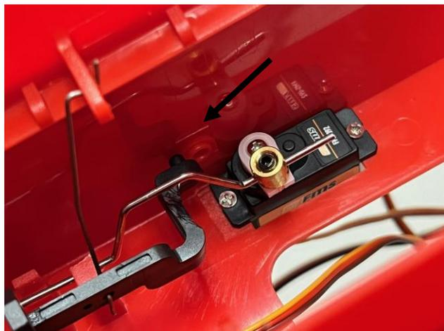
*The pin that holds the nose gear mechanism in place had popped out during shipping. It was an easy fix but a good lesson to check over all parts of a plane before flying.*
