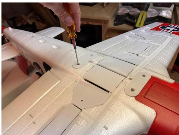
*Only four screws and two plastic brackets hold the wings onto the fuselage. Two wing spars held to add rigidity to the wings*
