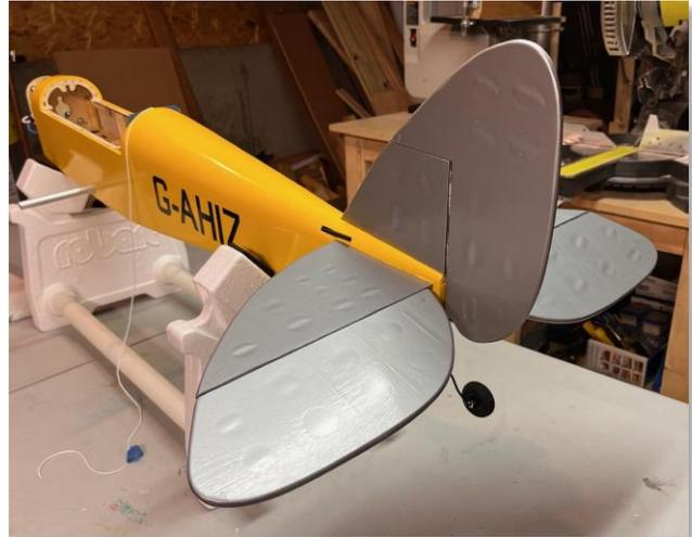
Horizontal and vertical stabilizers installed. The fiberglass hinges had to be glued in place and the control arms were set with epoxy.
