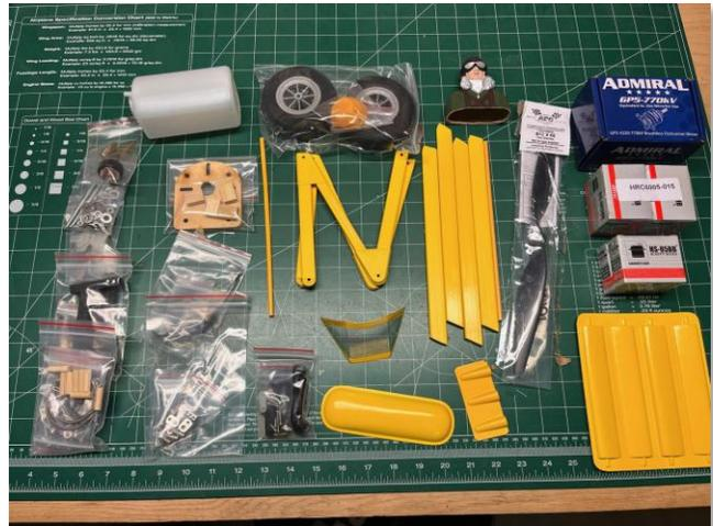
Lots of bits and pieces to put together. An Admiral motor and Hitec servos were used for this build.
