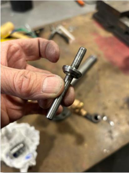
*Exhaust valve after silver soldering and machining*
