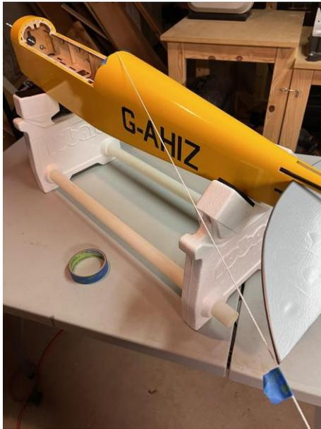
Aligning the horizontal stabilizers.
