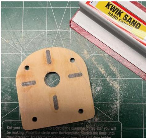
Mounting plate holes filled with epoxy and sanded smooth so they can be drilled through later.
