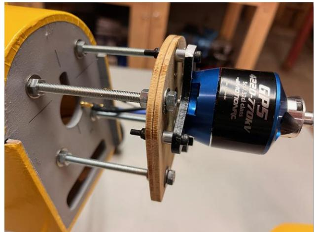
Aluminum spacers were added to mount the motor to the motor mounting plate to achieve the necessary 130 mm length from the firewall to the opening of the cowl.
