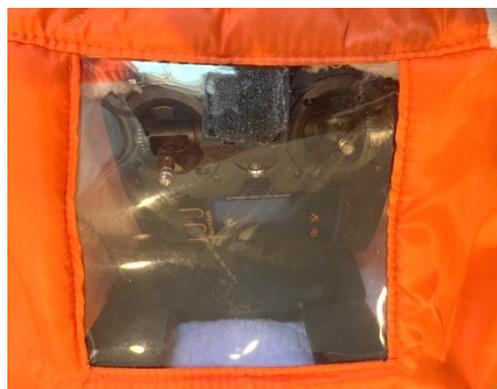
**Transmitter and foam platform is visible through the window. Notice the space for a hand warmer**
