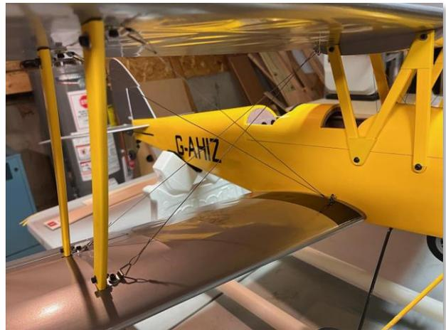
Guy wires were attached to the upper and lower wings on both sides of the plane. They added a nice touch of realism. Having a crimping tool made securing the wires a breeze.
