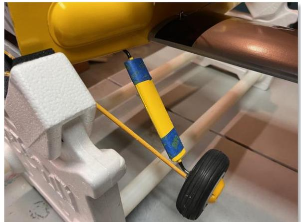
The two halves of the landing gear covers were attached to the metal gear using silicone glue and temporarily held in place with tape. A plastic yellow straw was used to cover the front gear wire.
