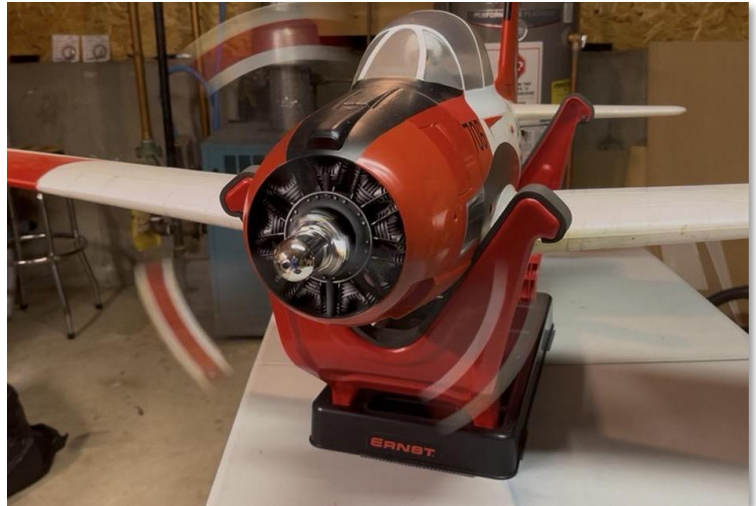
The repaired motor, prop and spinning all reinstalled that the loud sounds are gone. All ready for the re-maiden flight.
