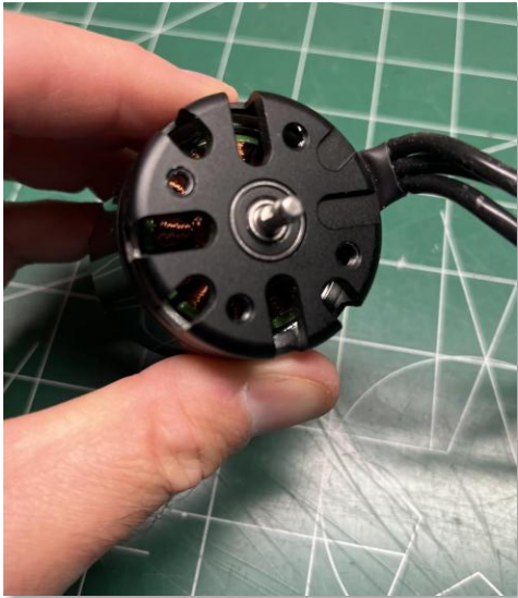
New sealed bearing installed on the T-28's motor.
